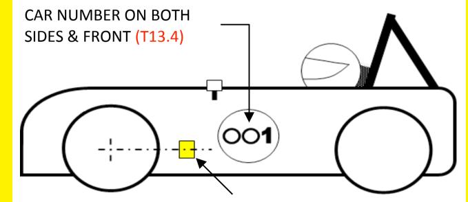
TRANSPONDER MOUNTED AT FRONT AXLE HEIGHT BETWEEN FRONT AXLE AND SIDE NUMBER (T13.5)
